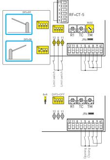
[Example 2]. Control N.C. 1-6 [safety stop] can be changed into control N.O. 1-4 [closing] setting  $6\rightarrow$ 4=0FF.
